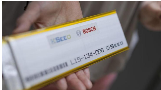
Prototyp of a new LiB with Lithium-Metal as electrode and a solid polymer as electrolyte
